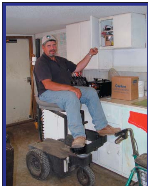
David Hofstetter demonstrating his custom scooter with elevating chair.
