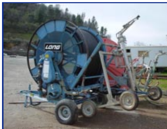
A traveling gun sprinkler allows Bernard to irrigate his crops without needing assistance to move an irrigation pipe.
