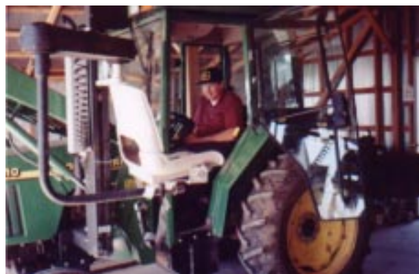
Dave Filer accesses his John Deere 5210 with a seated Pilot Lift from Life Essentials.
