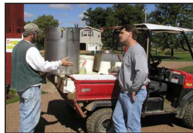
Purvis explains how an old water heater he mounted to the Kawasaki Mule makes for easy hauling of water and milk replacer to the calf hutches.
