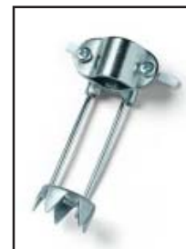
Five Cleat Ice Pick for Canes: This plated steel attachment has five points to prevent a cane or crutch from slipping on snow-covered, slushy, or icy surfaces. It clamps onto canes from 5/8" - 1" diameter.
