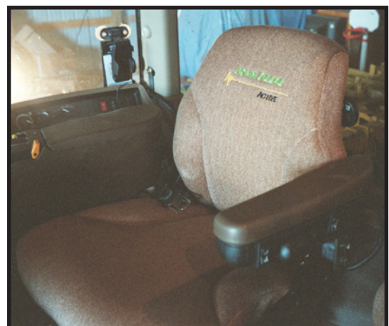
Anderson's new "Active Seat" has a vibration dampening system, which reduces stress on his ligaments and nerves.
